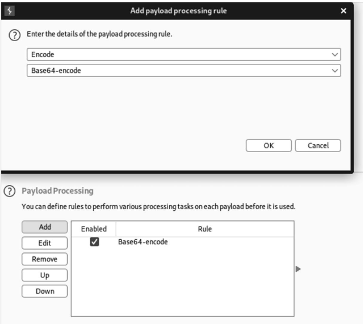
Figure 8-6: Adding a payload-processing rule to Burp Suite Intruder
