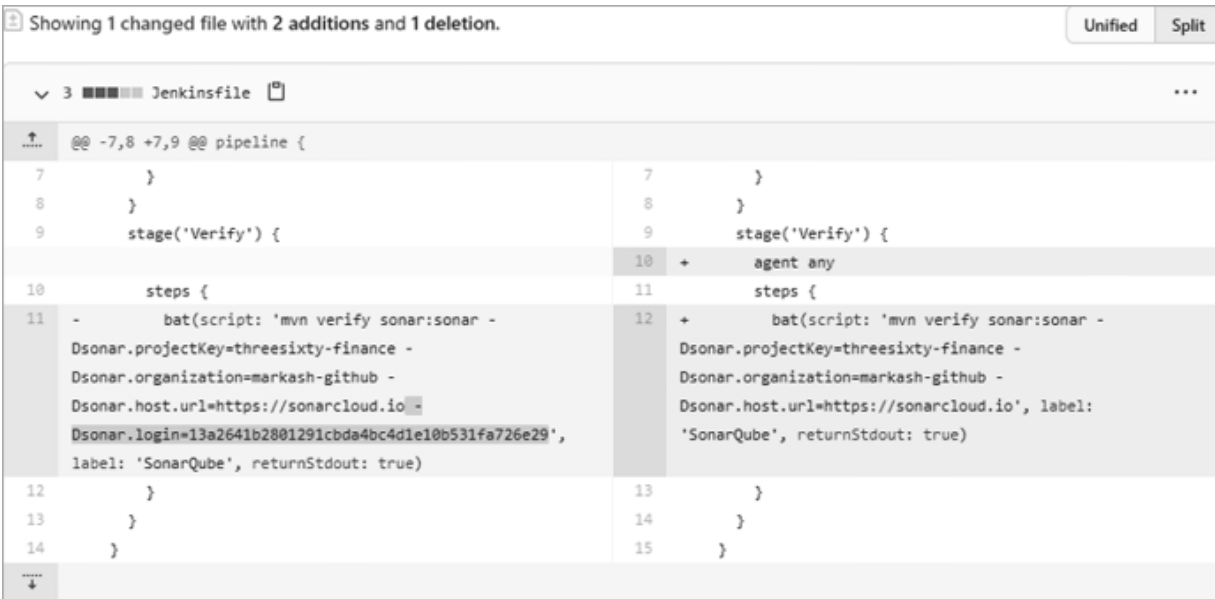
Figure 6-8: The Split button allows you to separate the previous code (left) from the updated code (right).
