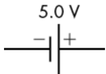
Figure 5-2: Circuit symbol for a 5-volt DC power source
