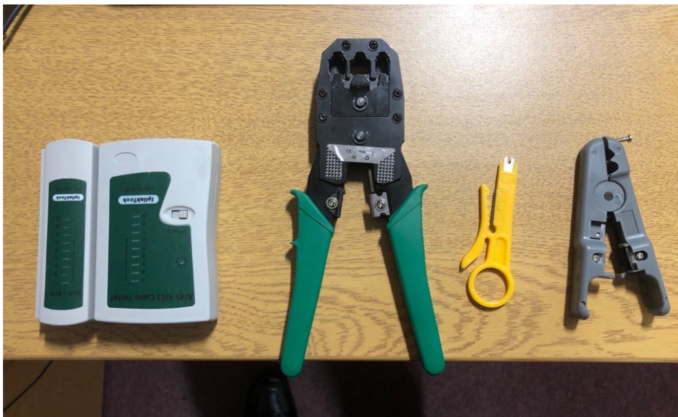
Fig 1. Cable preparation tools. R-L Cable tester, Crimping tool, rotary cutter, alternate rotary cutter (only one type in each kit)
